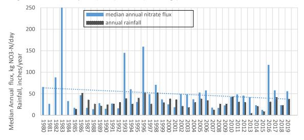
Figure 2-25: Summer Nitrate Concentration, San Lorenzo River at Big Trees Median annual nitrate concentration at Big Trees monitoring station (060) between 1980 and 2019 in comparison to annual rainfall. Monitoring data from the City of Santa Cruz. Rainfall data are from the California Irrigation Management Information System (CIMIS), site 104 (De Laveaga). The dark horizontal line represents the target nitrate concentration (mg/L as N)
