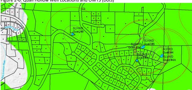
Figure 2-6: Quail Hollow Well Locations and OWTS (Dots)
