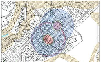
The Altivo well is to the north and the Sells well to the south. Inner buffer is 150 ft and outer buffer is 600 ft. Black dots are parcels with OWTS.
